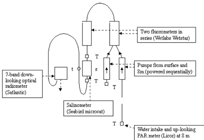
Fig 3. Pumped water flow in the sensing system used on buoy 46134. "T" indicates small flow-through anti-fouling modules. The outflow water is pumped onto the window of the radiometer to discourage growth.
