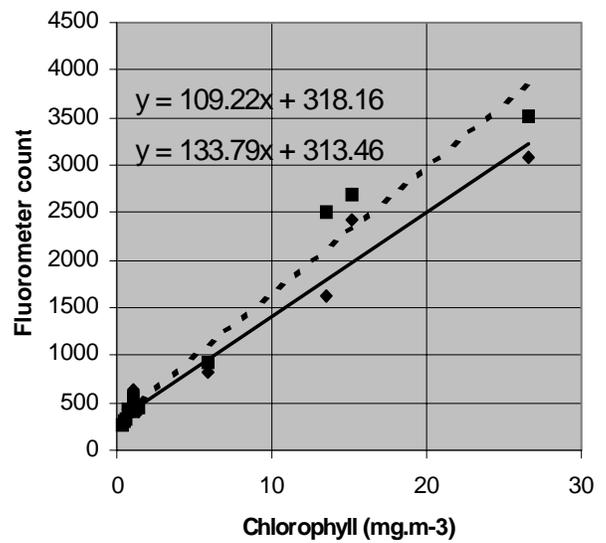
Fig. 7. Calibration of the two fluorometers using results of analysis of water samples from 8-meters depth.
