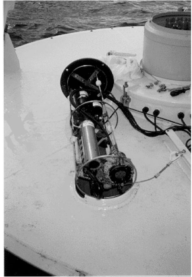
Fig. 2b. The "biological" instrument package withdrawn from the well in which it is mounted to look below the buoy. The lower end of the package is closer to the camera, over the well opening. Instruments presently include two fluorometers, a salinometer, and a 7-band optical radiometer. An optical PAR meter and a deep water inlet are hung 8 meters below the package.
