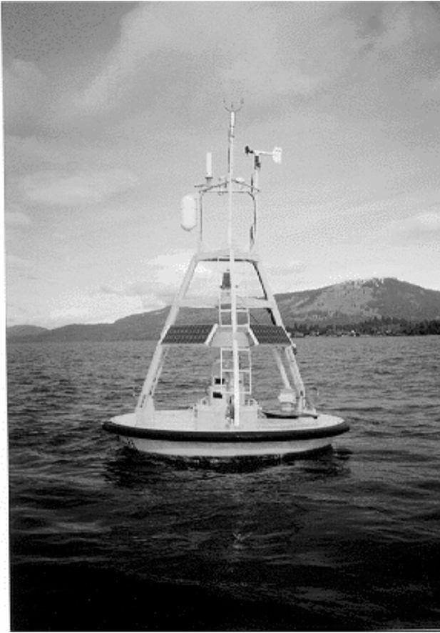
Fig. 2a. Weather buoy 46134 in Saanich Inlet near IOS. The buoy design is based on a standard 3-meter discus hull. Anemometers, radar reflector and satellite antennae are mounted at about 4 m above the sea surface. An automatic water sampler is mounted on the centre of the buoy deck. The top of the package holding the optical instruments can be seen on the deck at right.
